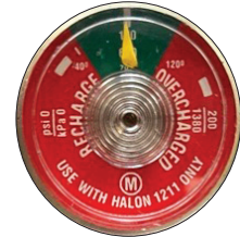
Halon Extinguisher Pressure Gauge
