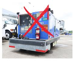
chemical types. The acidic properties of monoammonium phosphate become increasingly reactive when exposed to moisture or humid environments. This enhanced acidity can result in pitting corrosion on certain untreated metal surfaces. This corrosion can be difficult to detect, especially within crevices or inaccessible areas of an aircraft. If left unidentified, such deterioration poses a significant risk, potentially leading to structural or electrical failures during critical moments.
