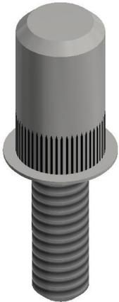
The rivet type stud is a ¼–20UN–2A threaded stud with approximately ¾” of length. This device may be used for mounting detector brackets, conduit fasteners, PRM clips, pipe hangers, etc. Attach devices to the stud using a standard ¼-20UN nut and lock washer. Rivet studs come 10 to a bag. UL listed.
