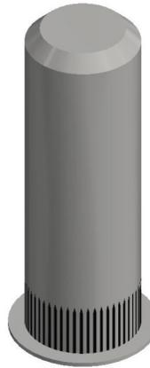
The rivet type nut is tapped ¼–20UN–2B with approximately ¾” of length. This device may be used for mounting detector brackets, conduit fasteners, PRM clips, pipe hangers, etc. Attach devices to the tapped blind rivet using a standard ¼-20UN bolt or screw and lock washer. Rivet nuts come 10 to a bag. UL listed.
