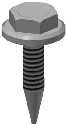
Quik-Fasteners are available for securing LHD Support Clips to a sheet metal mounting surface. These fasteners are supplied 24 to a bag along with a pilot drill bit for easy installation using a hand drill (capable of 2000-3500 rpm) with a 10 mm hex driver. These fasteners are self sealing. Installation instructions are provided with each bag. UL listed.
