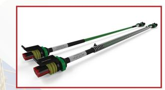
Linear Heat Detection cables have long been the industry standard and provide a continuous heat detection cable that runs inside the hazard area. The Amerex Advantage has amped up the traditional cable with a more robust abrasion resistant outer jacket and factory-installed connectors for reliability and ease of service. The cable is also available with a stainless steel wire protective covering for extreme environments.
