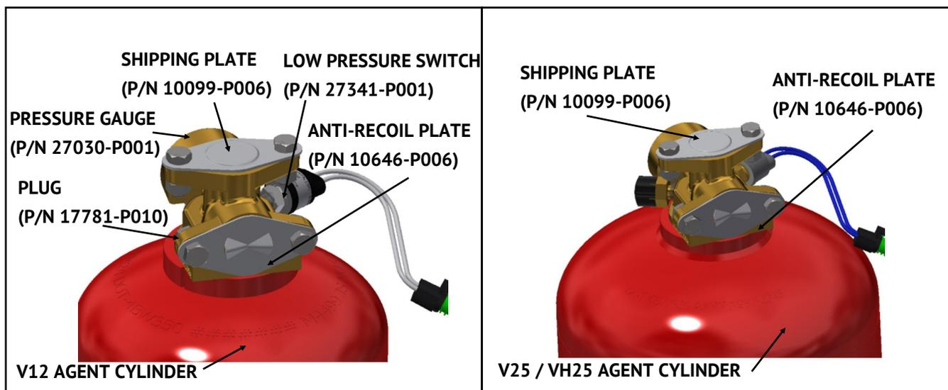
The Amerex ACT™ System agent cylinders are available in two sizes, with different mounting options and orientations. There are two different types of agent cylinders, those for use in total flooding applications and those for use in local applications. All agent cylinders are shipped fully charged from the factory. All agent cylinders are specialized DOT 4BW350 cylinders, tested to 700 PSI (4826 kPa). The operating temperature range of the cylinders is -40°F to 120°F (-40°C to 49°C).
