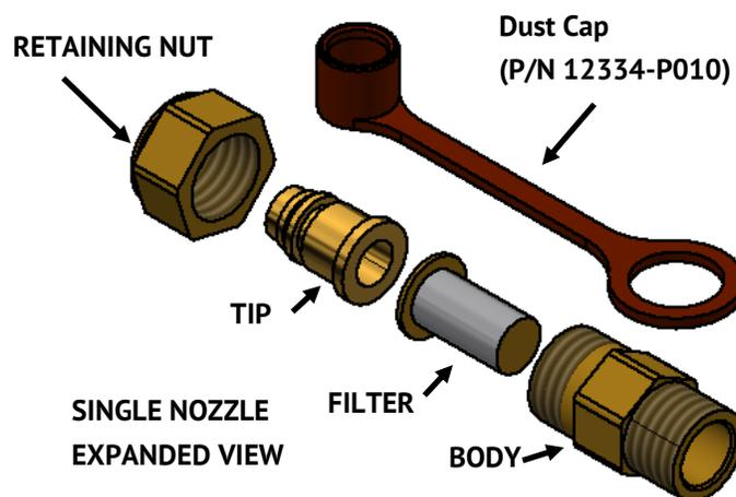
Three (3) different types of nozzles are offered for use with the ICS system as shown in the table below. Each nozzle has a specific full cone pattern diameter and range for dispersing the ICS agent to the hazard area. For specific nozzle ranges, see figure below. All nozzles used in the system are supplied with filters. All nozzles are also supplied with dust caps to prevent contamination from entering or blocking the nozzle tips. Replacement dust caps are available (P/N 12334-P010).
