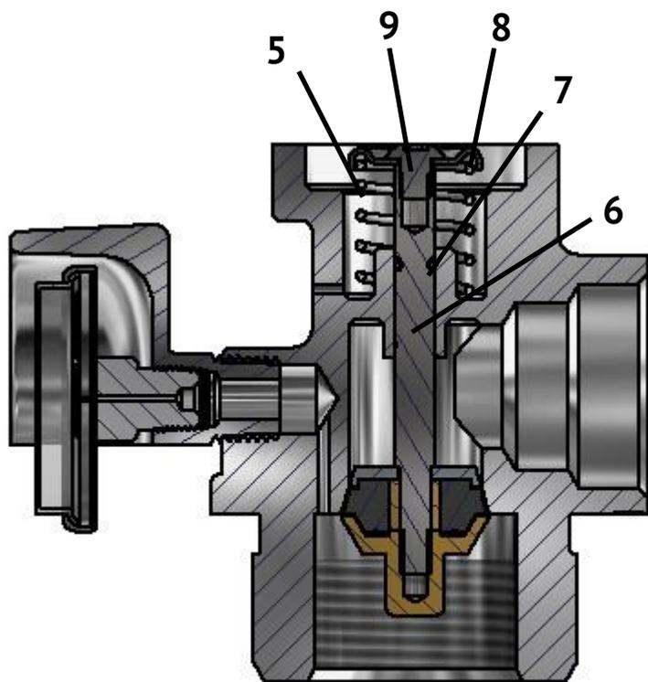
The Cylinder Valve Assembly is made with forged brass. The valve stem is made of stainless steel. The valve has a 350 psi pressure gauge protected by a gauge guard. The valve controls agent discharge via a spring loaded, internal sealing valve stem that must be depressed from the top of the valve either by pneumatic actuation or electrically by utilizing a Linear Actuator and Electric Control Head.
