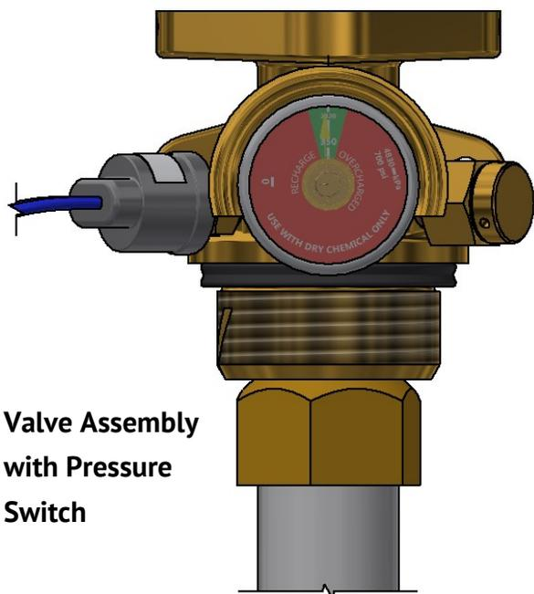
Valve Assembly with Pressure Switch
