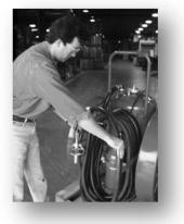
Adjust the loops so that the nozzle fits into the nozzle mount. Loops should be approximately the same size.
